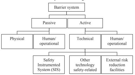
Fig. 2. Schematics of classification of safety barriers [17]
