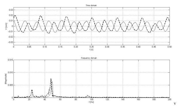
Fig. 4. Waveform and frequency spectrum of engine vibration velocities for jacked up idle running car, solid line is for car with engine equipped with supercharger
