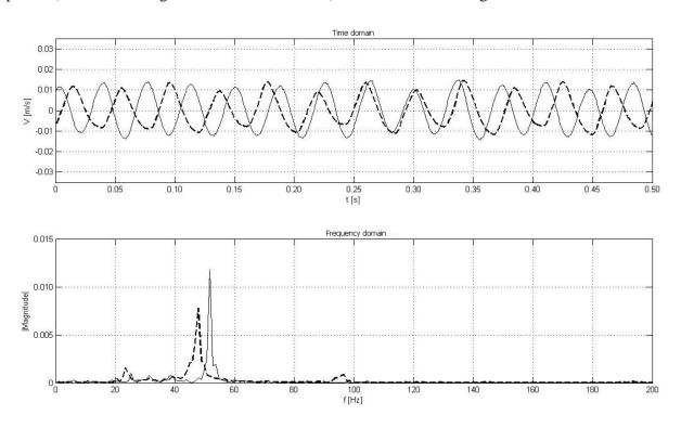
Fig. 3. Waveform and frequency spectrum of engine vibration velocity for not jacked up idle running car, solid line is for car with engine equipped with supercharger
