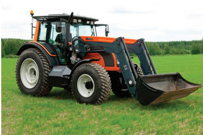
Fig. 6. Valtra N101 AGCO tractor, fuelled with biogas
