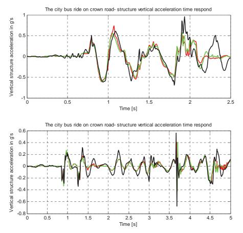
Fig. 7. Structure vibration accelerations time respond with tree different force-velocity characteristics of damper element while riding on two different road profiles (crown upper one and polyline lower one)
