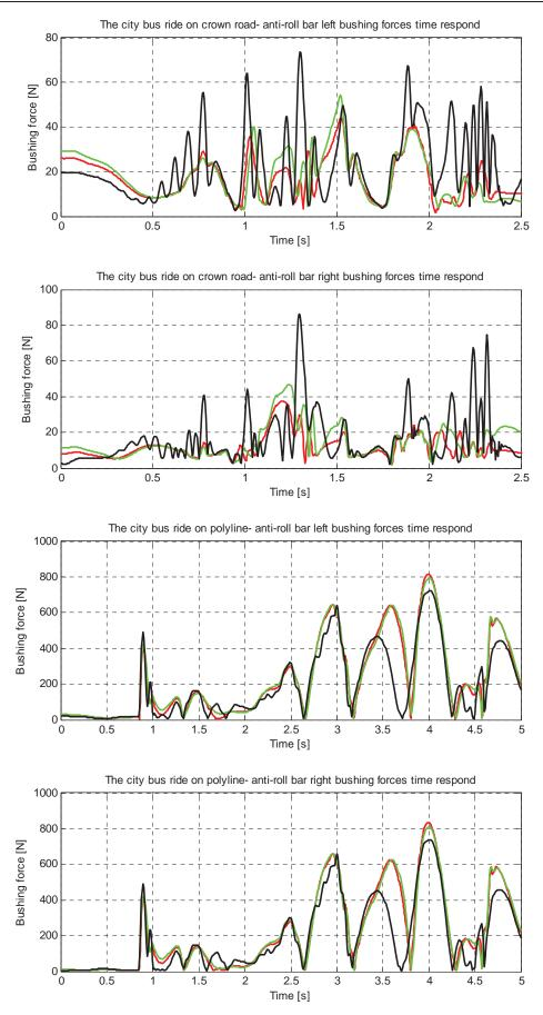
*Fig. 6.* Anti-roll bar bushing force time respond with tree different force-velocity characteristics of damper element while riding on two different road profiles (crown upper one and polyline lower one)
