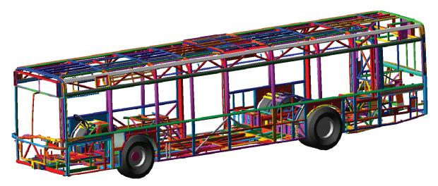
Fig. 2. The multibody model of the city bus
