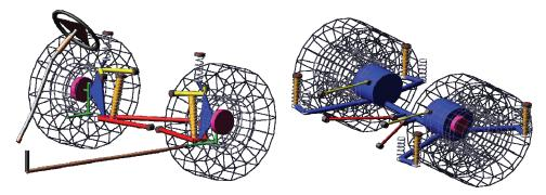
Fig. 3. Front and rear suspension models of the city bus
