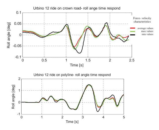
Fig. 5. Roll angle time respond with tree different force-velocity characteristics of damper element while riding on two different road profiles (crown upper one and polyline lower one)
