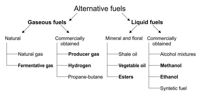
*Fig. 1. Division of alternative fuels used to power internal combustion engines* [2]
