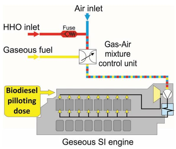
Fig. 2. Diagram of connection generator to the engine when the gas is feed to inlet manifold
