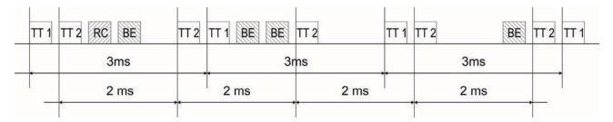
Fig. 5. Partitioning time between TTEthernet messages
