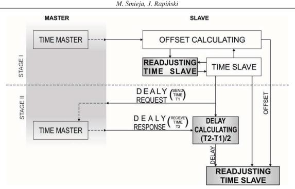
Fig. 2. Example of PTP synchronization
