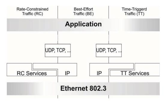
Fig. 6. Relation of TTEthernet to existing communication Standards [16]
