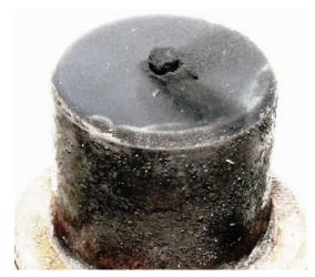
Fig. 4. View of injector hole pintle nozzle coking field of CFR engine for Cetane number determination (O&GI Cracow)
