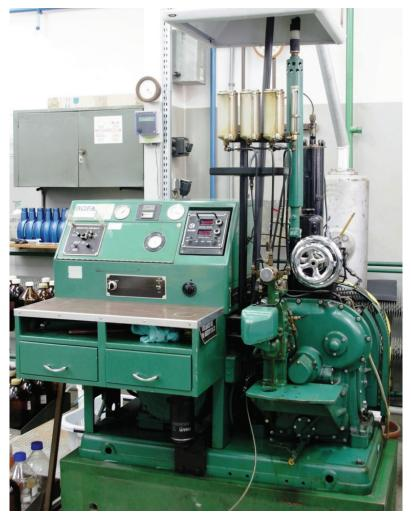
*Fig. 1. View of CFR Waukesha engine test bed for Cetane number determination according to ASTM D 613 (O&GI Cracow)*
