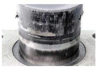
Fig. 5. Carbon deposit on piston crown and piston skirt of manual setting wheel for change of test engine combustion chamber volume (O&GI Cracow)
