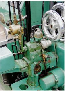
Fig. 2. Single-assembly fuel injection pump of CFR Waukesha engine for Cetane number determination according to ASTM D 613 (O&GI Cracow)
