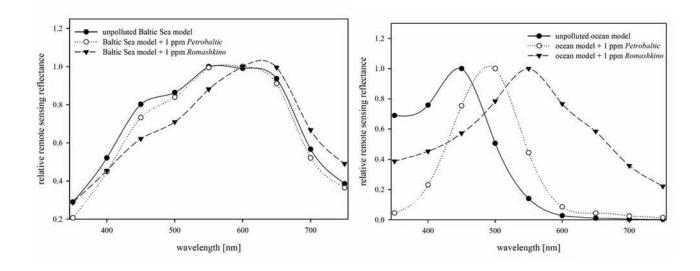
Fig. 4. Examples of relative remote sensing reflectance spectra (shapes are comparable)
