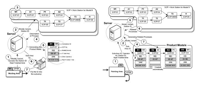
Fig. 9. An initialization mechanism at the product model Fig. 10. Development of sub-model of a product at construction monitoring point CP-02
