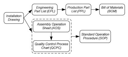
Fig. 2. Engineering processing in utilizing product installation drawing
