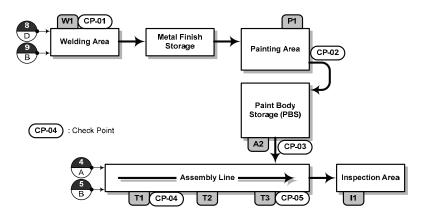
Fig. 8. An example of the monitoring point location design
