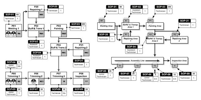
Fig. 5. Relation among SOP model with production Fig. 6. Mapping of standard operation procedure to process sequences a production unit
