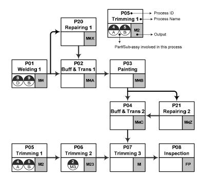
Fig. 4. Model of process which shows sequence of production process
