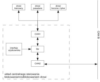
Fig. 2 Schematic diagram of system of selective door locking
