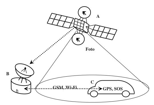
Fig. 1. Principle of operation of the SOS system
