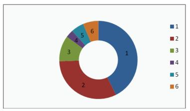
Fig. 1. Causes of fires in engine rooms where: 1 – fuel systems - 40%, 2 – lubricant oil systems – 30%, 3 – electrical systems - 10%, 4 – turbo compressors and exhaust gases piping -3%, 5 – waste oil systems (incinerating plants)-5%
