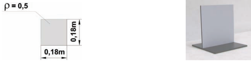
Fig. 2. Target for visibility research by means of STV method on pedestrian crossing
