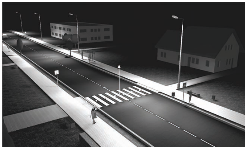
Fig. 5. Pedestrian crossing illuminated by lighting frames
