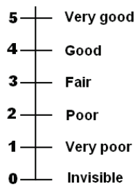
Fig.3. Visibility level VL by means of STV method
