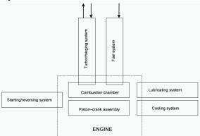
Fig. 1. Engine division into functional sub systems
