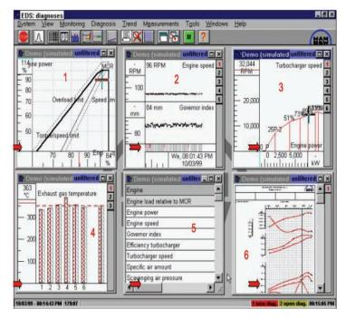
Fig. 3. Monitoring parameters In CoCoS-EDS module. 1 - engine running area with current running point, 2 – engine speed and load factor time graph, 3 – turbocharger speed in the function of engine horse power, 4 – exhaust gases temperatures on particular cylinders, 5 – values of selected engine parameters, 6 – general engine characteristics
