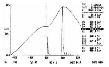
Fig. 5. Pressures recorded in cylinder and the vibrations curves with the use of GNU indicator
