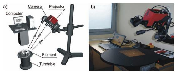
Fig. 1. The measuring system GOM ATOS: a) schema, b) photography
