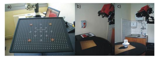
Fig. 3. Measurement with the rotary table: a) calibration, b) turntable calibration, c) measurements of gear
