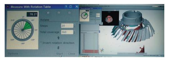
Fig. 4. Measurement pinion using the rotary table – data processing
