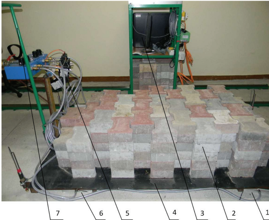
Fig. 1. Object of study: 1, 6 – air pads, 2 – load, 3 – data acquisition and control system, 4 – platform, 5 – proportional valves, 7- handle
