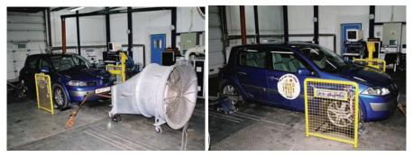
Fig. 4. Chassis dynamometer stands
