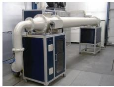
Fig. 7. Dilution exhaust gases device
