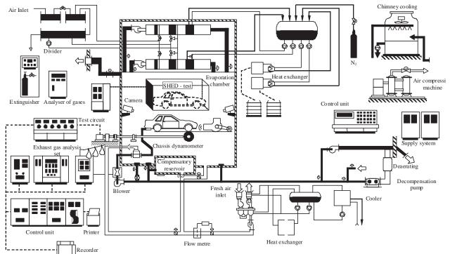
Fig. 6. Scheme of chassis dynamometers stand
