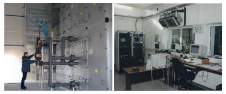
Fig. 5. Temperature chamber and chassis dynamometers stand control devices
