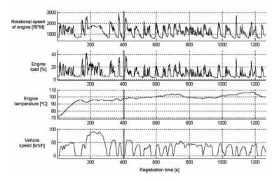
*Fig. 2. Vehicle performance record during FTP75 test on chassis dynamometer, implementation of oxygen sensor monitor marked with vertical line, RPM, engine loading [%], engine temperature [*<sup>0</sup>*C*]*, speed [km/h]*
