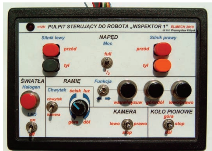
Fig. 6. Built wire control panel
