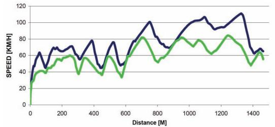
Fig. 5. Characteristics of speed in the function of the path, for the fastest and slowest driver in the test (blue fast driver, green slow)
