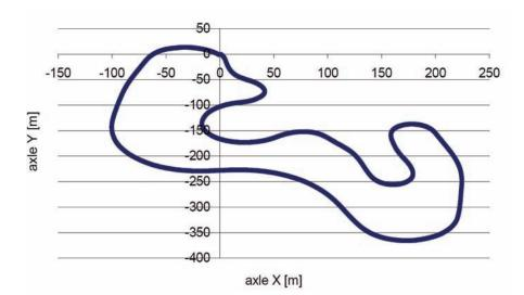
Fig. 7. Geometry characteristics of the go-kart loop on the Poznan Track in the square coordinates of the measurement system
