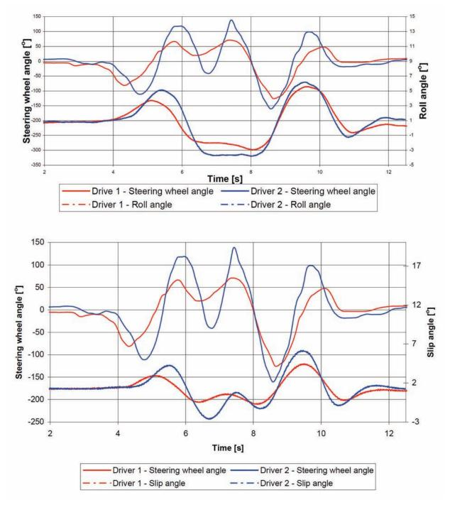
Fig. 8-10. Characteristics of the steering wheel angle along with: lateral acceleration, angle of slip and drift in the function of time for the two drivers
