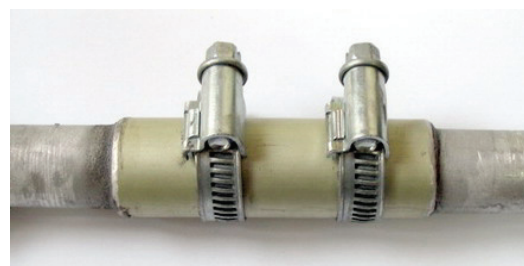
Fig. 6. The method of achieving pressure during bonding
