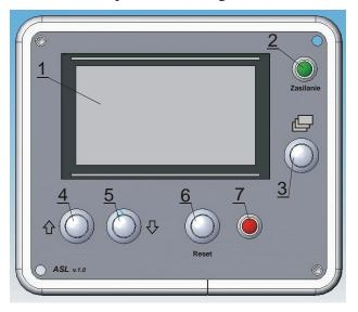
Fig. 5. General view of the ALS v 1.0 control panel: 1 – LCD display; 2 – power-on diode indicator (green); 3 – panel key for switching between system screens; 4 – panel key for scrolling the screen up; 5 – panel key for scrolling the screen down; 6 – Reset key; 7 – fault diode indicator (red)
