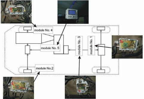
Fig. 3. Location of actuating modules in the Tarpan Honker vehicle
