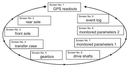
Fig. 4. Hierarchical structure of ALS screens
