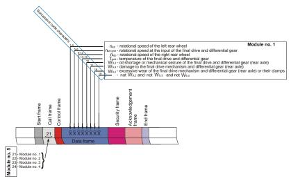
Fig. 2. Principal structure of the data protocol generated by module No. 1
