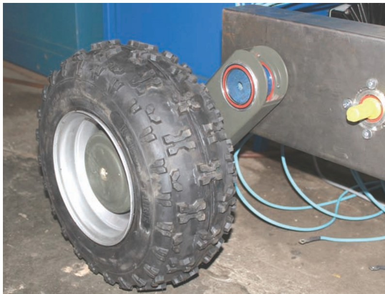
Fig. 8. Rocker arm and wheel assembled on the UGV frame
