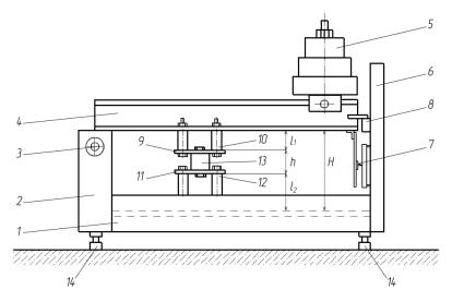
Fig. 1. Vibration isolators' test bench scheme
