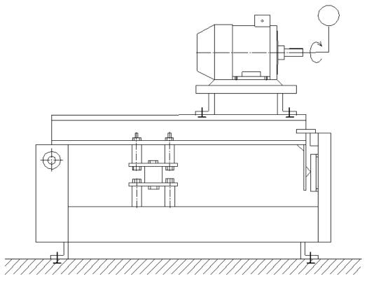
Fig. 7. Scheme of forced oscillations excitation system on the test bench by inertial exciter
