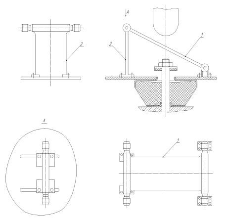
Fig. 5. Design of the device for loading the vibration isolator with vertical and lateral loads combination
