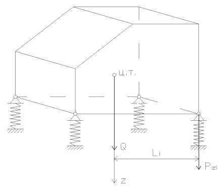
Fig. 4. Scheme of vibration isolators installation in the real technical object's suspension
