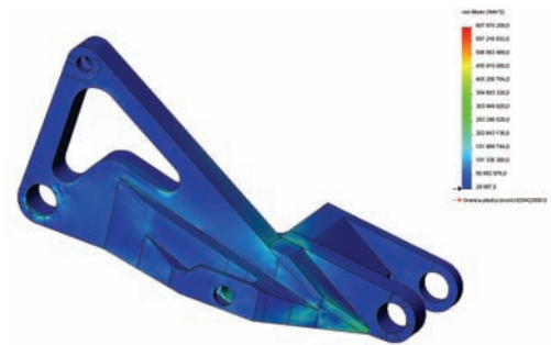
Fig. 21. Layer model during Finite Elements Method strength calculations
