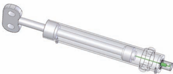
Fig. 10. LS2 hydraulic cylinder mounted to the body
