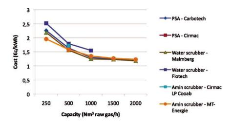
Fig. 1. Estimated cost of biogas upgrading plants using different technologies [3]
