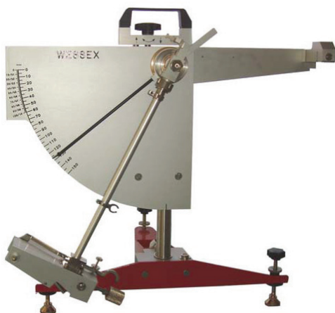
Fig. 2. Examples of portable measuring devices, used to assess the road surfaces skid resistance in the process of its supervision and technical maintenance [6,7]
