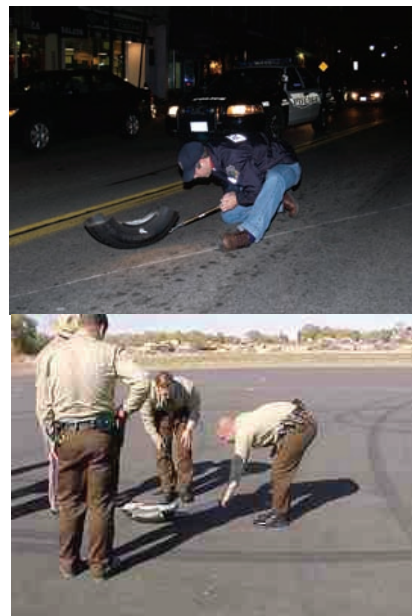
Fig. 3. Examples "drag sleds" used to assess road surface skid resistance in place of road accident [8,13]
