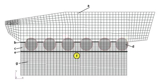
*Fig. 6. Scheme of analyzed vehicle: a – hull, b – ALE coupling surface, c – air area, d – wheels, e – border of two domains, g – ground, f – explosive*
