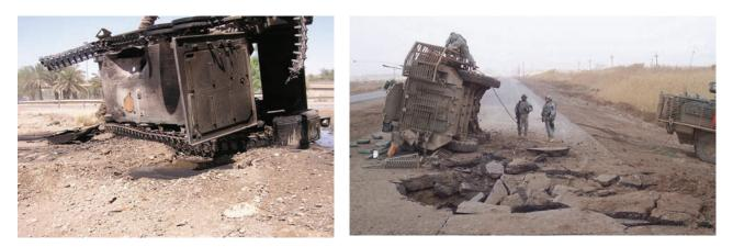
Fig. 1. An example of IED detonation under different vehicles [US ARMY photo]
