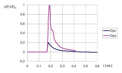
Fig. 4. Comparison of pressure impulse of free wave Dpc and reflected wave Dpo for 125 g TNT charge
