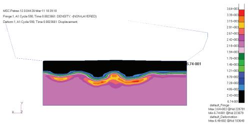
Fig. 11. Pressure distribution through right side section of the vehicle for the time t = 0,00236 s
