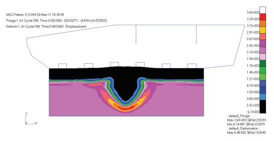
Fig. 10. Pressure distribution trough the symmetry plane section of the for the time t = 0.00236 s
