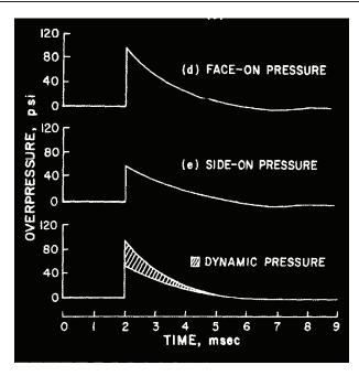
Fig. 3. Static and dynamic pressure for near ground explosion [D. R. Richmond 1970]
