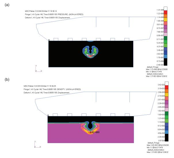
Fig. 9. Pressure distribution trough section of the vehicle (a), ground and air density (b) for the time t = 0.00051 s
