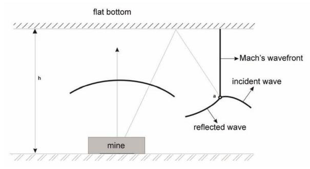
Fig. 2. Wave reflection from vehicle's bottom
