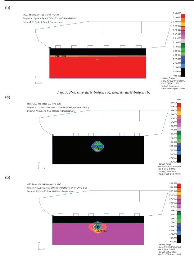
Fig. 8. Pressure distribution trough section of the vehicle (a), ground and air density (b) for the time t = 0.00022 s
