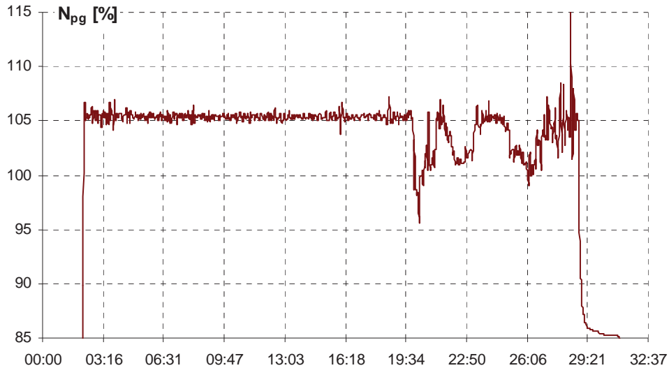
Fig. 7. Waveform for rpm variations of the helicopter rotor and the driving turbines for the both engines
