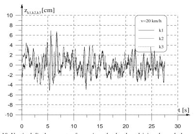
Fig. 10. Vertical displacements of carrying wheels when driving through the ground
