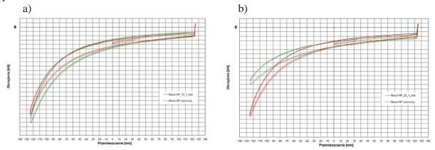
Fig. 11. Elastic characteristics of hydro-pneumatic suspension components along with the characteristics of the master: a) functional element, b) faulty item
