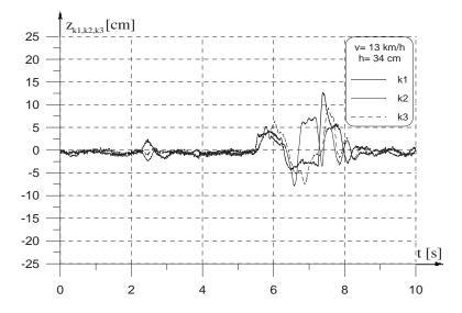
Fig. 8. Vertical displacements of carrying wheels sequentially
