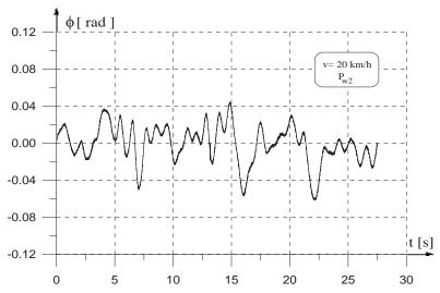
Fig. 9. Angular movements of the hull of the CV when driving through the ground
