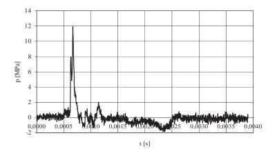
Fig. 13. Distribution of pressure acting on a selected area of the bottom of the hull
