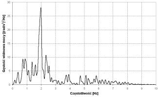
Fig. 14. Power spectral density estimator of tank gun vibration
