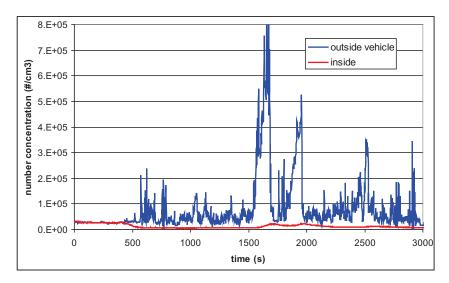
Fig. 9. Particle concentration inside and outside a passenger car with the filter turned on. Even when the external concentration is extremely high, in this example while driving through a tunnel, the indoor concentration remains very low
