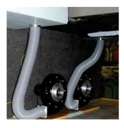
Fig. 13. Filter system for buses, installed in the luggage compartment
