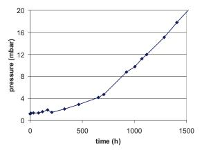
Fig. 5. Filter pressure drop as function of operating time in a highly polluted road tunnel
