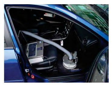
Fig. 7. Filter, particle sensor (below notebook) and Notebook for data acquisition
