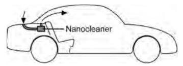
Fig. 6. One possible solution to mount the filter system
