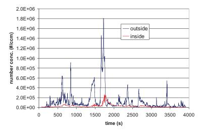
Fig. 12. Particle concentration inside and outside of the truck cabin
