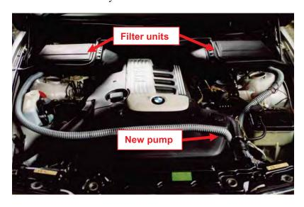
Fig. 15. The original filter of the BMW 530 has been replaced by high efficiency filters. Air is supplied by a blower, which is also placed in the engine compartment
