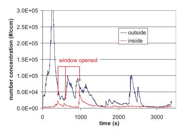
Fig. 14. Particle concentration inside and outside a coach. Three times, indicated by the red arrows, a window has been opened. Immediately the indoor concentration rises to approach the outdoor concentration and decreases again after the window is closed
