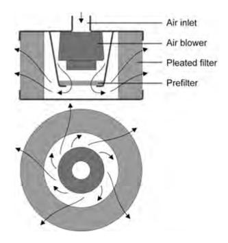
Fig. 3. Setup of the filter with integrated prefilter for course particles and blower
