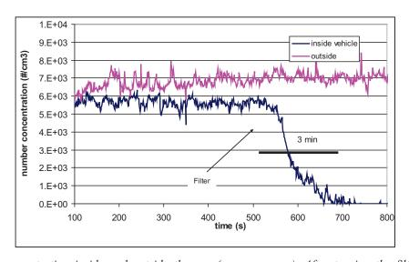
Fig. 8. Particle concentration inside and outside the car (passenger car). After turning the filter on, the inside concentration drops to very low levels over about three minutes
