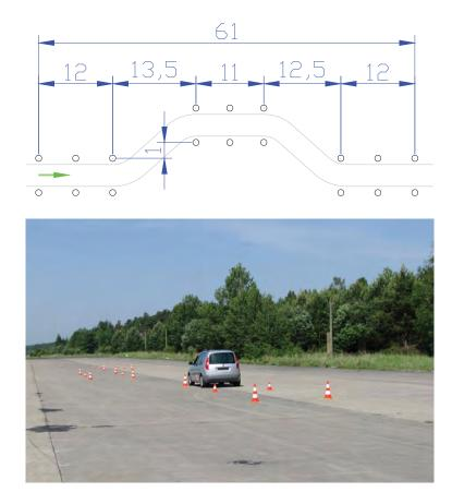
Fig. 1. Test VDA ISO TR 3888 – top view: track of the test (size in the meter), under view: Škoda Roomster during tests on the airport Hradčany-Mimoň
