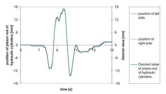
Fig. 3. Test VDA ISO TR 3888 on the testing bench - position of piston rod of hydraulic cylinders for supposed speed 60 km/h, sampling rate for control system 100 Hz, load for wheels 4.5 kN, tyres 15"
