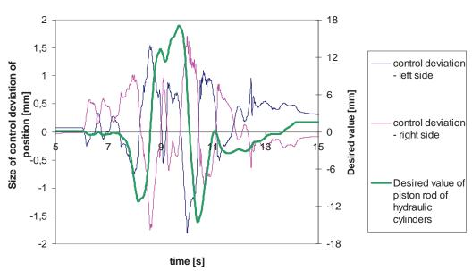
Control deviation positions of piston rod of hydraulic cylinders
