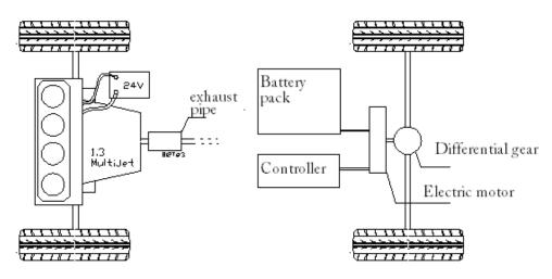
Fig. 1. Prototype hybrid powertrain layout
