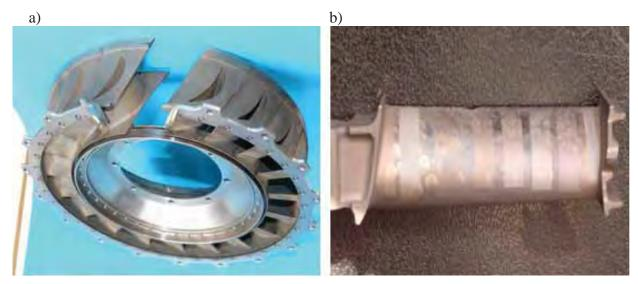
*Fig. 1.* The studied elements of aircraft turbine engine: *a*) the turbine blades before cleaning, *b*) turbine blade lasercleaned in the laboratory conditions
