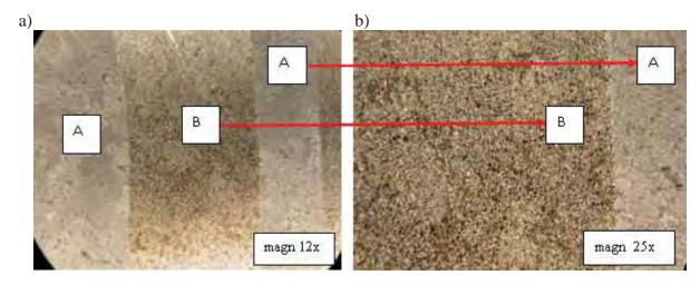
Fig. 6. Jet engine turbine blade made (cast) of nickel based alloy WI ŻS6K purified by the use of the laser: A - greasy surface, B - purified surface by the use of the radiation of pulsed Nd: YAG laser with power density  $q = 1.53 * 10^6$  W/cm2, and scanning speed v = 5m/s
