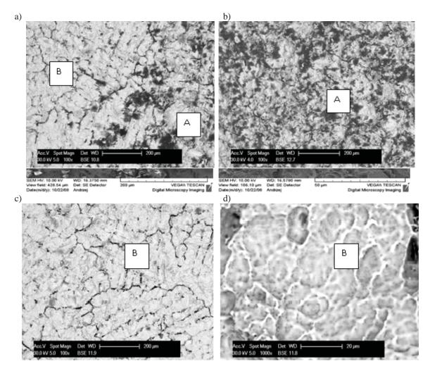
*Fig. 3. Characteristic area of the surface layer of heat resistant nickel alloy* ŻS6K-WI after casting and laser ablative *cleaning:* A - a zone before cleaning, B - a zone after cleaning
