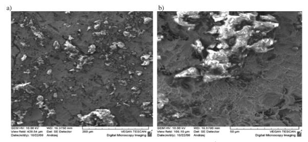
Fig. 2. The characteristic surface topography of heat resistant nickel alloy ŻS6K-WI used in the manufacture of turbine blades of aircraft engines - the material after casting
