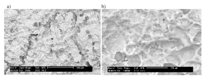
Fig. 4. Characteristic area of the surface layer of heat resistant nickel alloy ŻS6K-WI after casting and laser ablative cleaning - apparent micro partial melting zones
