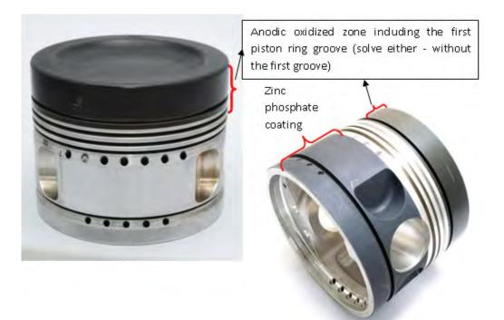
Fig. 2. Production piston engine UTD-20
