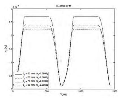
Fig. 4. In-cylinder mass of air in the function of crankshaft rotation angle for the examined inlet pipe diameters at rotational speed of 2200 1/min
