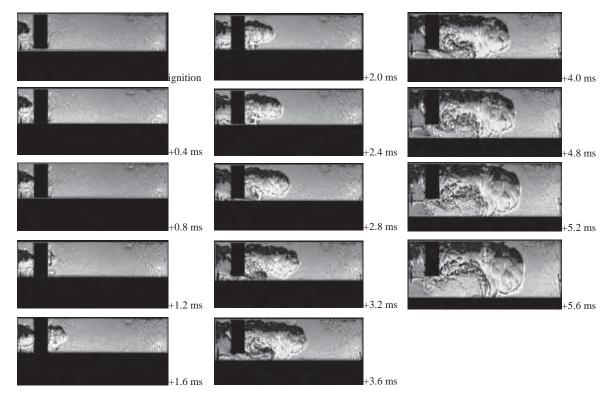
Fig. 2. Course of combustion in RCM for system configuration:  $V_{kw}=10\%$ , d=3mm, ignition in the prechamber centre,  $\varphi_{wz}=20^{\circ}$  CAD BTDC
