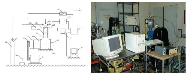
Fig. 1. Schematic and view of RCM test stand
