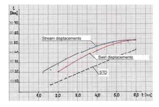
Fig. 5. Flame front travel versus time for the situation presented on Fig. 4
