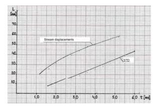
Fig. 3. Flame front travel versus time for the situation presented on fig. 2
