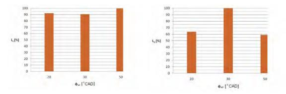
Fig. 7. Comparison of compression work  $(L_s)$  and effective work  $(L_u)$  of RCM for ignition advance angle: 20° CAD, 30° CAD, 50° CAD BTDC (System configuration  $V_{kw}=10\%$ , d=3 mm, ignition in prechamber centre)
