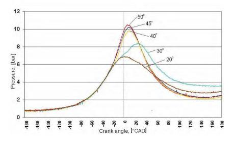
Fig. 6. Comparison of pressure courses in RCM combustion chamber for different ignition advance angles: 20° CAD, 30° CAD, 50° CAD BTDC (System configuration  $V_{kw}=10\%$ , d=3 mm, ignition in prechamber centre)
