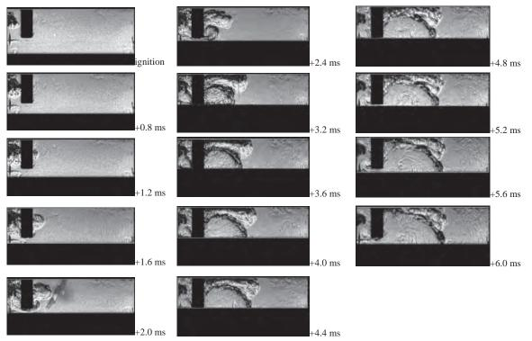
Fig. 4. Course of combustion in RCM for system configuration:  $V_{kw}=10\%$ , d=3mm, ignition in the prechamber centre,  $\varphi_{wz}=50^{\circ}$  CAD BTDC
