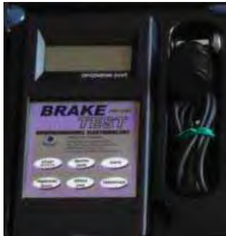
Fig. 3. Decelometer - Brake Test LWS-2MC with acceleration sensor
