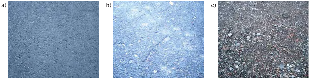
Fig. 4. Surfaces on which measurements were made – a) new asphalt, b) destroyed asphalt, c) gravel
