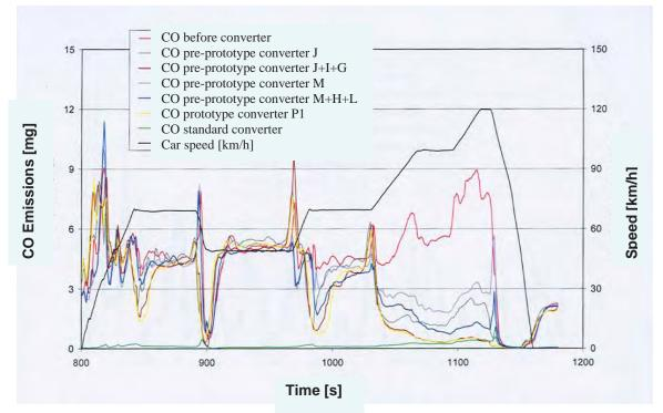
Fig. 5. CO emissions in the EUDC phase of the NEDC test for FIAT Panda 1.3 Multijet with different versions of catalytic converters
