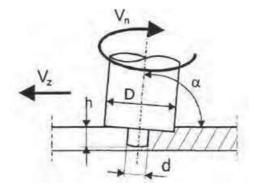
Fig. 1. The diagram of FSW
