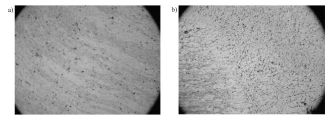
Fig. 4. Microstructures of joint: a) welded by FSW, b) welded by MIG
