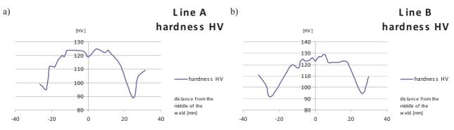
Fig. 2.Hardness distribution of FSW welded joints: a) near the surface, b) in the middle of the specimen
