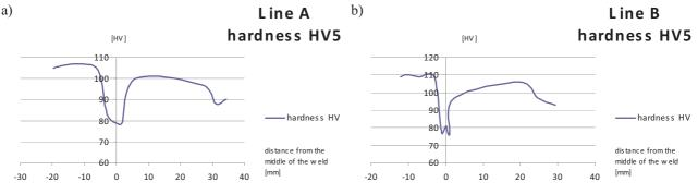
Fig. 3. Hardness distribution of MIG welded joints: a) near the surface, b) in the middle of the specimen
