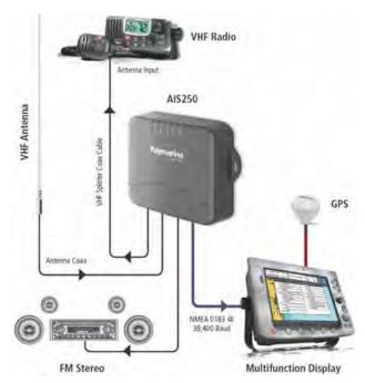
Fig. 2. AIS configuration [2]
