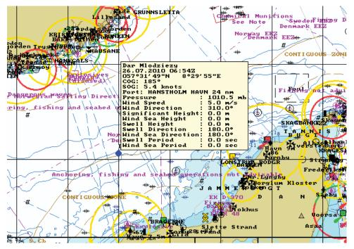
Fig. 3. Example information obtained with AIS [1]
