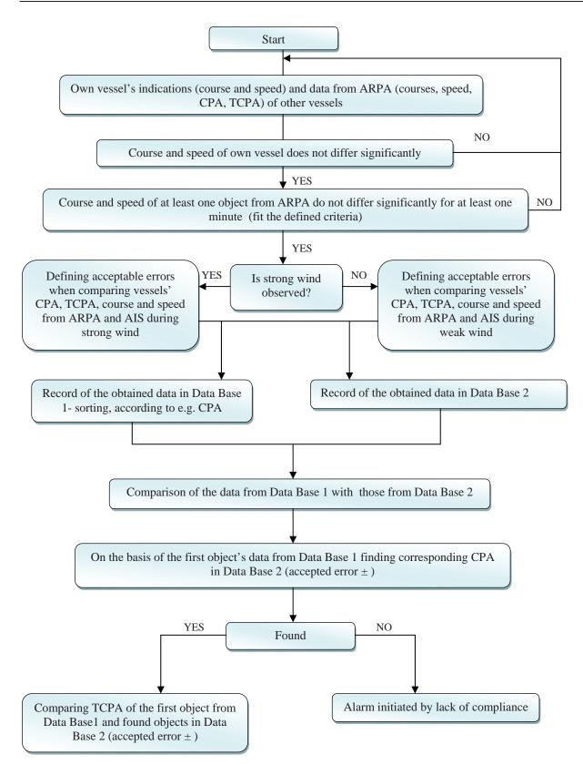
Fig. 5. Example algorithm for finding errors of ARPA and AIS indications
