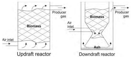
Fig.2. Scheme of updraft and down draft gasifier
