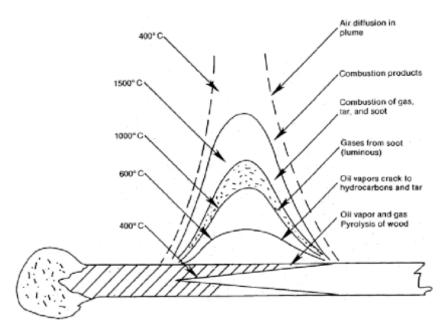
Fig. 1. Pyrolysis, gasification and combustion processes in flaming match [3]
