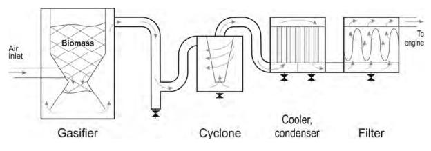
Fig. 4. Typical gas conditioning setup
