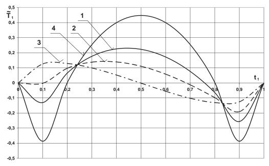
Fig. 5. Change the dimensionless friction forces  $\tilde{T}_1$  in the time  $t_1$  by velocity perturbations: 1)  $V_{10}$ =0.05,  $V_{1h}$ =0,005,  $V_{1h}$ =0.05,  $V_$
