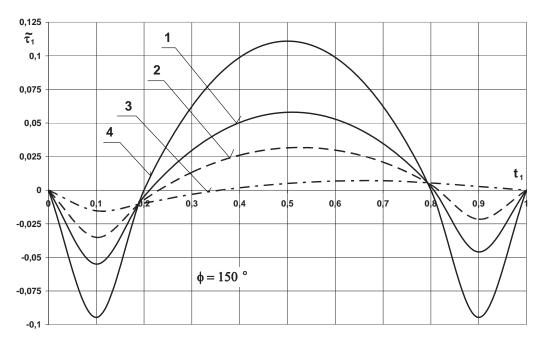
Fig. 4. Tangential pressure distributions  $\tilde{\tau}_1$  in place  $\varphi = 150^{\circ}$  in the time  $t_1$  by velocity perturbations: 1)  $V_{10} = 0.05$ ,  $V_{1h} = 0.05$ ,  $V_{1h} = 0.05$ ,  $V_{1h} = 0.025$ , 3)  $V_{10} = 0.05$ ,  $V_{1h} = 0.05$
