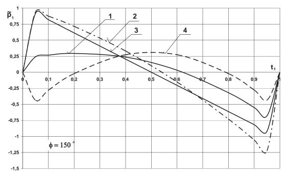
Fig. 1. Pressure distributions  $\tilde{p}_1$  in place  $\varphi = 150^{\circ}$  in the time  $t_1$  by velocity perturbations: 1)  $V_{10} = 0.05$ ,  $V_{1h} = 0.0$
