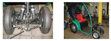
Fig. 6. Suspension with swivel axle [4]
