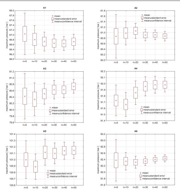
*Fig. 3. Representativeness of the mean maximum pressure depending on the number of averaged measurement cycles in the states of engine operation analyzed*
