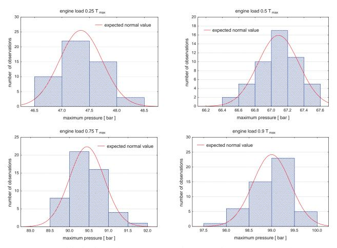
Fig. 1. Histograms of the distribution of maximum pressure values registered over 50 consecutive cycles for rotation speed 2500 rpm and respectively different engine loads
