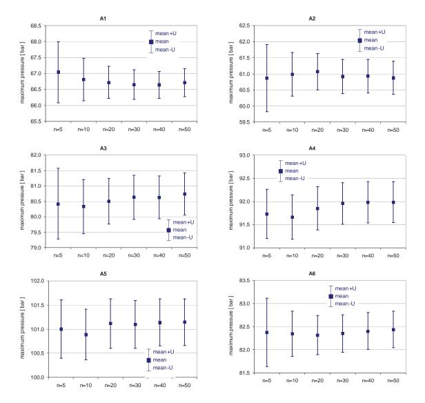
Fig. 4. Values of expanded uncertainty of the result of measurement in analyzed states of engine operation depending on the number of measurement cycles averaged
