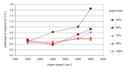
Fig. 2. The CV coefficient of variation for 50 pressure measurements performed for different engine operation states
