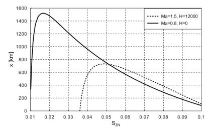
Fig. 1. Influence of the parameter of engine adjustment to the aircraft  $S_{ZN}$  on the theoretical range for the subsonic flight (full line) and supersonic flight (broken line)
