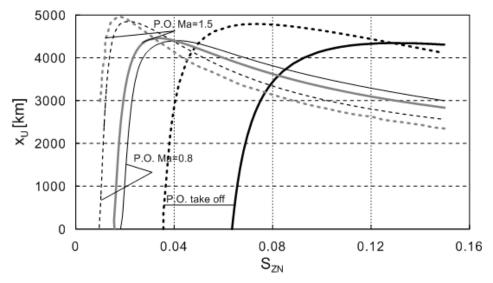
*Fig. 3.* Influence of choice of engine calculation point and S<sub>ZN</sub> on the conventional range of aircraft performed for Ma=1.5 H=5000 (full line) and Ma=1.5 H=18000 (broken line)
