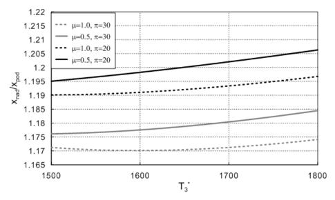
Fig. 7. Influence of temperature  $T_3$  and  $\mu$  as well as  $\pi$  for the relative range  $x_{pod}/x_{nad}$ . Subsonic flight Ma=0.8, supersonic flight Ma=1.6, H=12000 m
