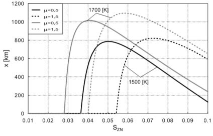
Fig. 5. Influence of bypass ratio  $\mu$  and temperature before turbine  $T_3^*$  and change SZN on the range x for the supersonic flight (Ma=1.6, H=18000 m)
