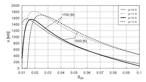
Fig. 4. Influence of bypass ratio  $\mu$  and temperature before turbine  $T_a^*$  and change SZN on the range x for the subsonic flight (Ma=0.8, H=0)
