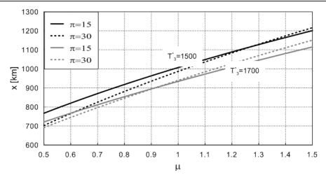
*Fig. 6. Influence of engine cycle parameters on the range x (subsonic flight)*
