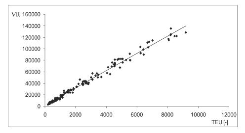
Fig. 4. Linear relation between container vessels displacement and container number (TEU)
