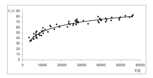
Fig. 3. Determination of proportionality factor (C) for ship's displacement in first range
