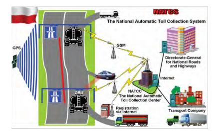
Fig. 2. The structure of the National Automatic Toll Collection System (NATCS)
