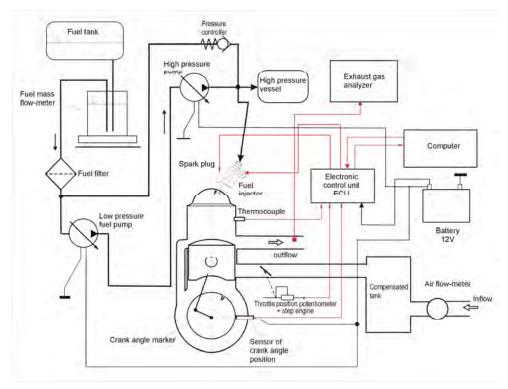
Fig. 1. Diagram of direct fuel injection two-stroke engine on experimental stand
