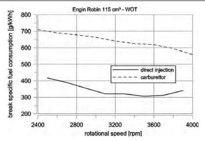
Fig. 4. Comparison of break specific fuel consumption of engine in carburetted version and direct fuel injection version
