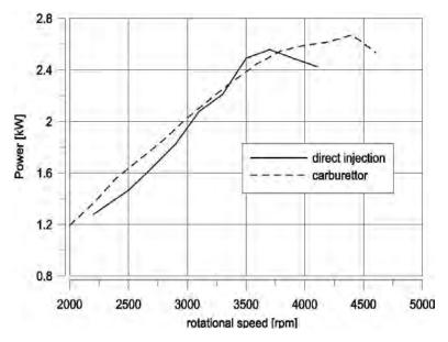
Fig. 3 Comparison of engine power in carburetted version and direct fuel injection version
