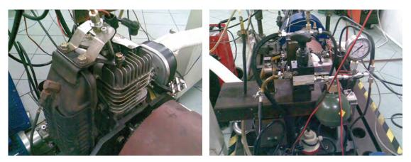
Fig. 2. Photos of experimental stand with direct fuel injection two-stroke engine
