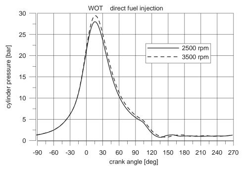
Fig. 8. Measured pressure traces in cylinder of direct fuel injection two-stroke engine at 2000 and 3000 rpm
