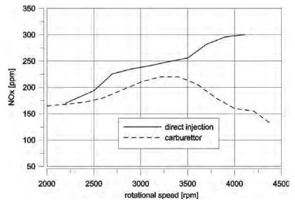
Fig. 7. Comparison of NOx volumetric concentration in exhaust gases in two-stroke engine for carburetted version and direct fuel injection version
