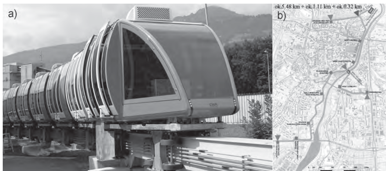
Fig. 3. Test monorail train manufactured by Bartholete (a), proposed train route (b)
