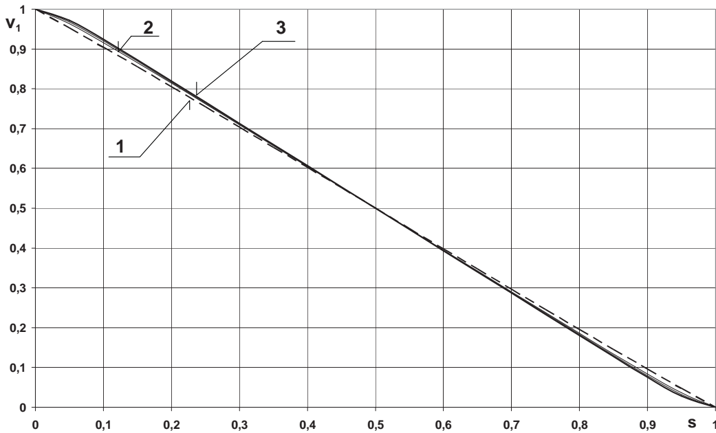
Fig. 4. Velocities V_1 in points of the maximal pressure of micropolar fluid \Lambda_1=20 : 1) N^2=0.1 , 2) N^2=0.5 , 3) N^2=0.9 from convergence coefficient \epsilon_{opt}
